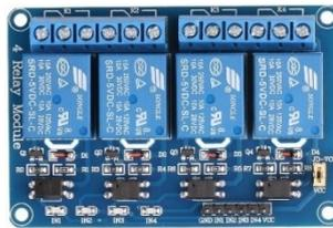
Gambar 4 Modul Relay 4 Channel
